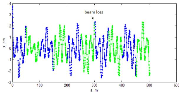
Figure 5: The betatron oscillations of injected beam obtained from the injection analysis. Only two kickers (BUIFB2 and BUIFB3) are operating at nominal settings. New turns start where the line colour changes. The initial s-coordinate corresponds to the injection septum exit on the first turn.
