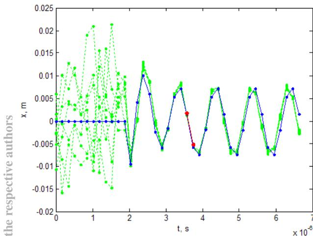
Figure 3: TBT BPM readings of the beam injected into the empty ring (green traces) taken over multiple injections. The noise up to the 12<sup>th</sup> turn ( $\approx 2 \mu s$ ) from beginning of the plot shows that there is no beam in the ring. Two red dots show the data we use to calculate the beam coordinates at injection point. The blue line shows the simulated trajectory of the beam injected with these initial coordinates.
