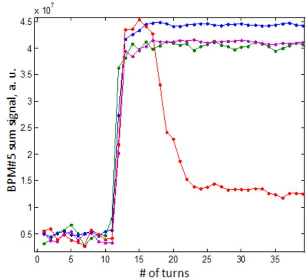
Figure 7: Sum signal of TBT BPM for the injected beam. Each point represents a BPM reading on a single turn. The injection is happening on the 12<sup>th</sup> turn. The green line represents the nominal 3-bump injection. Red line is two bump injection with BUIFB1 off. The magenta line is the modified two bump injection with increased BUIFB2 amplitude. The blue line is two bump injection with optimised settings of BUIFB1 and BUIFB3.
