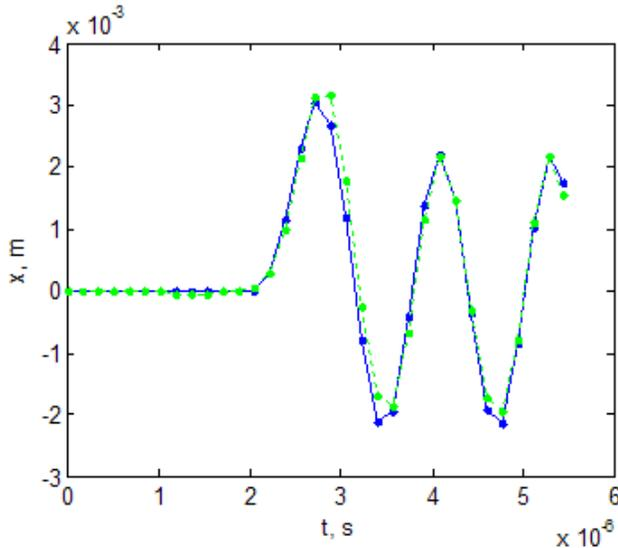
Figure 2: The oscillations of the stored beam kicked by BUIFB1 as read by TBT BPM #5 (green trace) and modelled (blue trace). Each dot represents BPM reading on a single turn.
