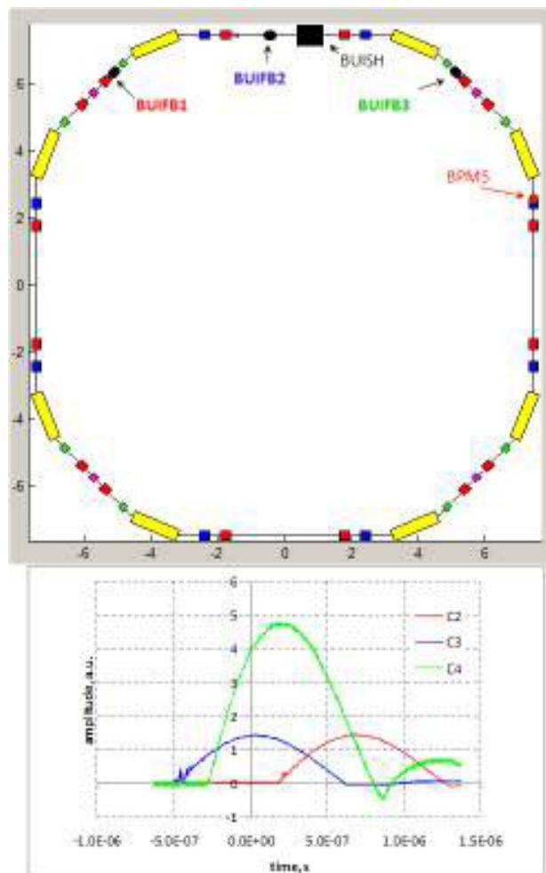
Figure 1: Locations of injection septum and fast injection kickers in the VUV ring (upper plot). The turn-by-turn diagnostics is connected to BPM5. Lower plot shows measured fast kicker waveforms in arbitrary units. Red line is BUIFB1, blue is BUIFB2 and green is BUIFB3.
