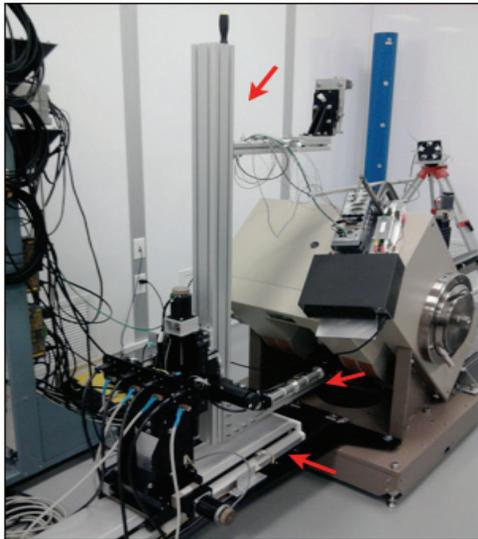
Figure 4: Hall probe supporting stage
