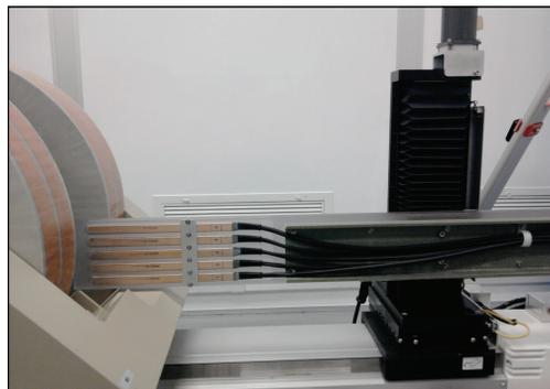
Figure 3: NMR probe supporting stage.
