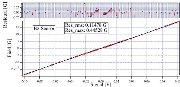
Figure 7: Calibration curve of Bz-sensor.
