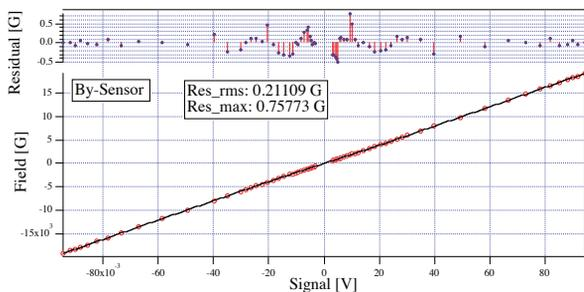
Figure 5: Calibration curve of By-sensor.
