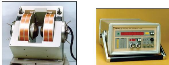
Figure 1: GMW dipole electromagnet and metrolab NMR teslameter.
