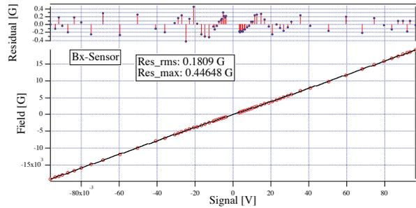
Figure 6: Calibration curve of Bx-sensor.
