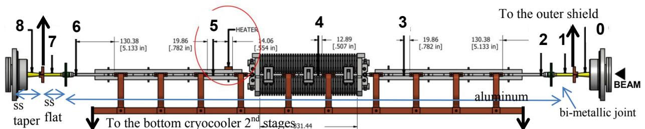
Figure 3: A schematic of the beam chamber, copper busbar, and locations of temperature sensors.
