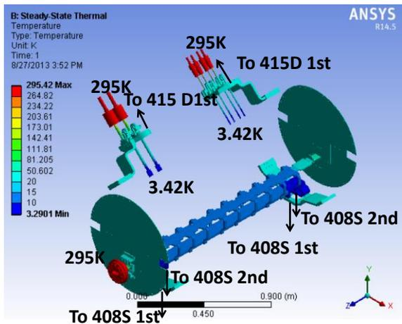
Figure 2: Calculated temperatures at the 20K and 60K circuits and their boundary conditions.
