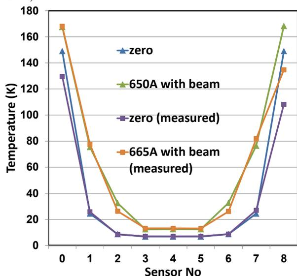
Figure 4: Calculated beam chamber temperatures are compared with measured temperatures.
