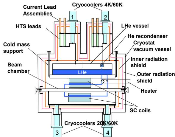
Figure 1: Cooling schematic.
