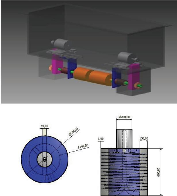
Figure 2: Schematic layout of the beam dump.
