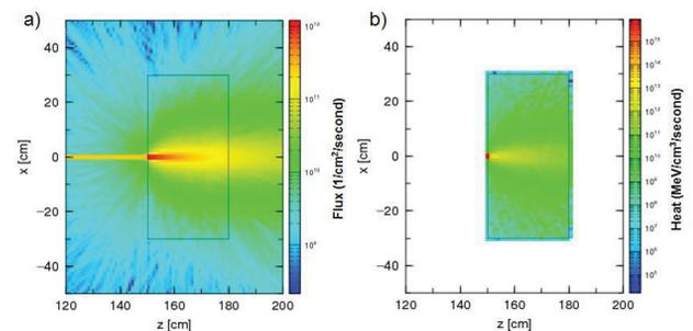
Figure 4: The distribution of the radiation flux (a) and the heat (b) on the beam dump.
