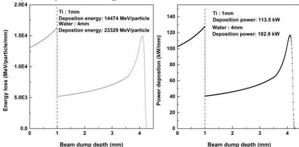
Figure 3: The energy loss (a) and the power deposition (b) of non-reacted <sup>238</sup>U beam at beam dump.
