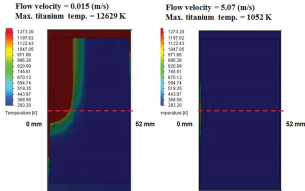
Figure 5: The temperature distribution in the beam dump due to absorption of 400 kW primary beams
