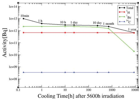
Figure 6: Activity of the beam dump as function of waiting time.
