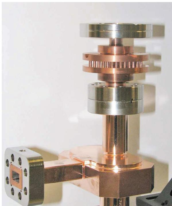
Figure 1: Metallic PBG structure and  $TM_{0,1}$  mode launcher at MIT prior to structure brazing. Note the open outer wall of the PBG cell.
