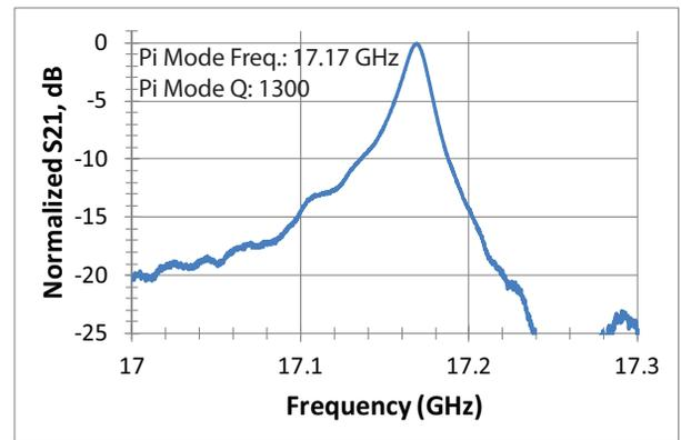
Figure 3: Transmission measurement of the second 17 GHz metallic PBG structure, prior to brazing. The Q of the mode of interest is found to be 1300 at a frequency of 17.169 GHz.
