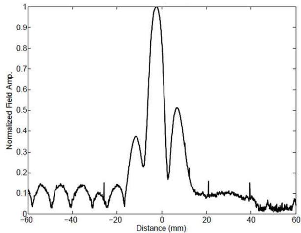
Figure 2: Measured field profile of first 17 GHz metallic PBG structure, obtained via use of a dielectric perturbation technique.
