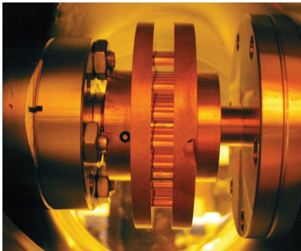
Figure 5: Metallic PBG structure installed in MIT test stand.
