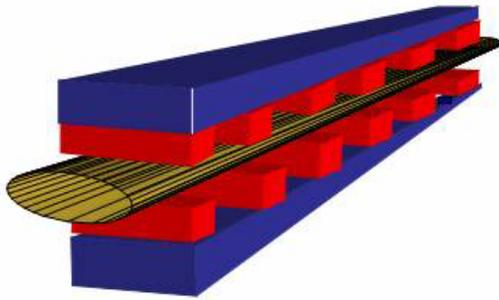
Figure 1: An elliptical cylinder, centered on the  $z$ -axis, fitting within the bore of a wiggler, and extending beyond the fringe-field regions at the ends of the wiggler.
