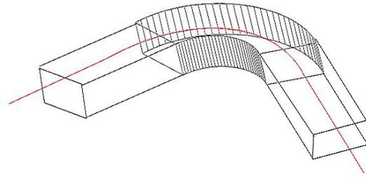
Figure 2: A bent box, fitting within a dipole, and having straight end legs that extend beyond the fringe-field regions at the entry and exit of the dipole.
