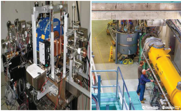
Figure 3: Photographs of the RF gun assembly used to produce first electrons (left) and of the cryomodule CM1 installation (right).
