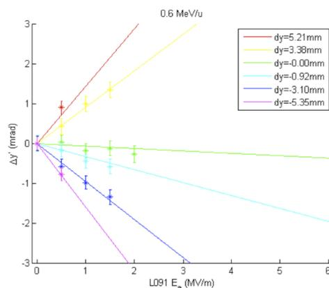
Figure 3: Vertical deflection angle vs. cavity voltage. Each line is the model prediction for different vertical displacement within the cavity from the beam's position. The diamonds including error bars represents the measured data.
