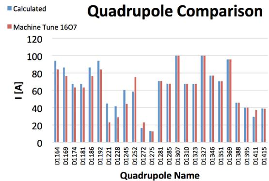
Figure 5: Comparison of quadrupole settings from machine model (blue) and as applied in machine (red).
