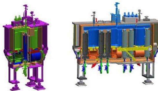
Figure 1: On the left the rebunching cryo module is shown with its cavity at the center between the solenoids. The right shows the first accelerating module with one cavity at each end and groups of two separated by the three solenoids.
