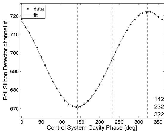
Figure 2: SRF cavity phase scan measured with a foil silicon detector. The dots represent the measured data, the line the fitted curve and the triangles with dashed lines, the location of maximum deceleration, zero crossing for the bunching slope and maximum acceleration.
