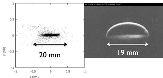
Figure 4: Transverse beam image in the location of a beam diagnostic station in the newly commissioned beam line. The left shows the simulated beam profile, the right the measured beam image.
