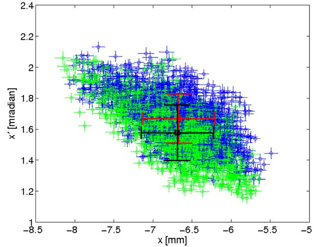
Figure 3: (Color) Horizontal injection offset measurement and the measurement distribution averages with one rms standard deviation from single-shot (blue, red) and LBEG+ (green, black) schemes.
