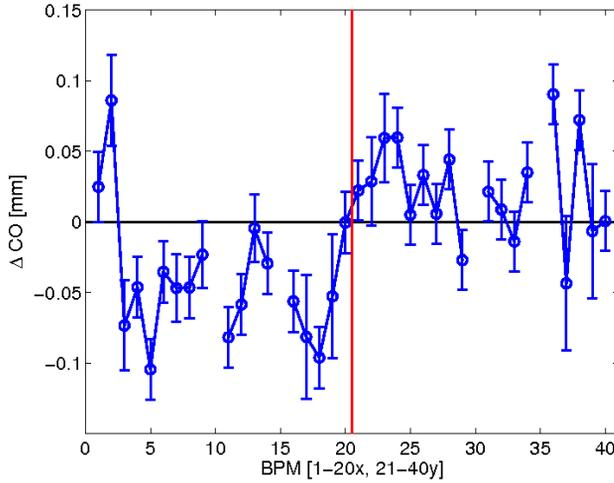
Figure 2: Difference in CO measurements using the single-shot and LBEG+ schemes with one rms uncertainty.
