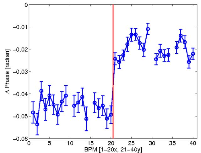
Figure 6: Difference in phase measurements using the single-shot and LBEG+ schemes with one rms uncertainty.
