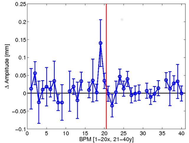
Figure 5: Difference in amplitude measurements using the single-shot and LBEG+ schemes with one rms uncertainty.
