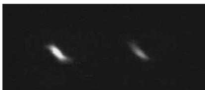
Figure 5: Image of two beams (corresponding to masses 76 and 77) as seen in the MCP viewer after the mass separator during one of the commissioning runs
