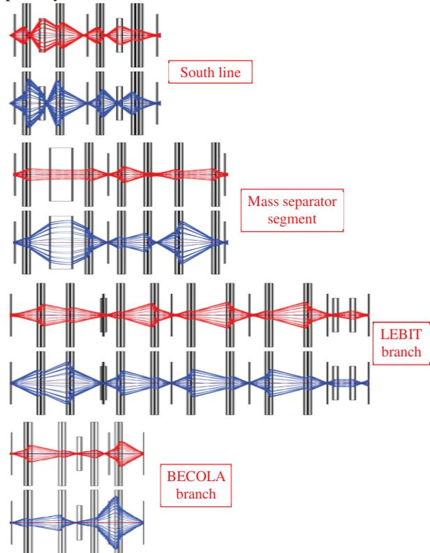
Figure 4: Ray calculations of beam transport in several segments of the line from South line to BECOLA (horizontal in blue, vertical in red)
