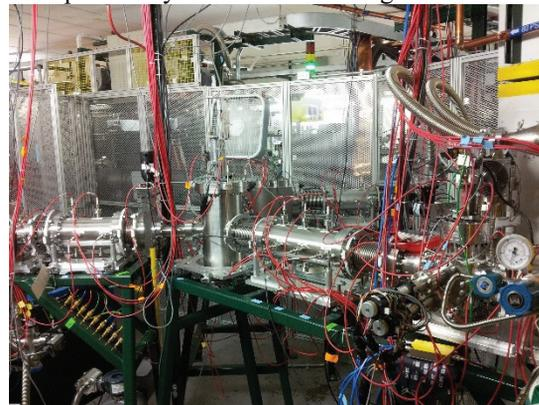
Figure 2: Merging point of the north and south lines. Starting from the left, the picture shows an electrostatic doubler, a bender and a triplet followed by the vacuum and diagnostic station before the mass separator.
