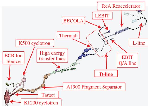
Figure 1: Layout of the CCF and ReA3 facilities (several high energy beam lines and experimental areas are not shown). The D-line connects the thermalization area with the low energy experimental hall and the charge breeder.
