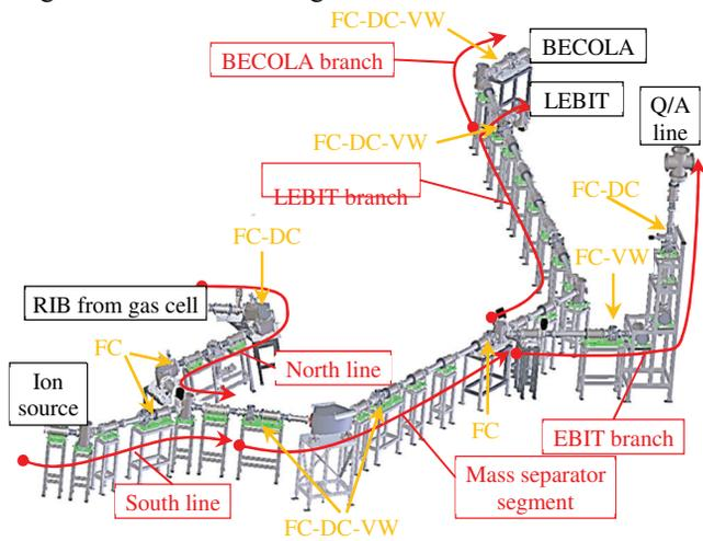
Figure 3: Layout of the D-line broken into different sections (in red), the beam origin/destination (in black) and a list of the diagnostics available at each location (in orange). FC stands for Faraday Cup, VW for MCP viewer and DC for decay counter.
