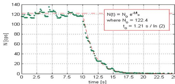
Figure 7: Decay curve for K-37 measured in the decay counter of the diagnostics station after the mass separator. The measured half-life is 1.21 s which is compatible with the expected value of 1.23 s.
