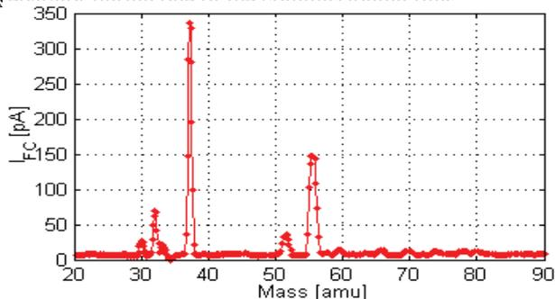
Figure 6: Mass scan during one of the Ga-76 commissioning runs. The different peaks correspond to different contaminant molecular beams produced in the gas cell as the high energy beam is slowed down and interacts with the residual gas. The two highest peaks correspond to mass 37 [H<sub>5</sub>O<sub>2</sub>]<sup>+</sup> and mass 55 [H<sub>7</sub>O<sub>3</sub>]<sup>+</sup>.
