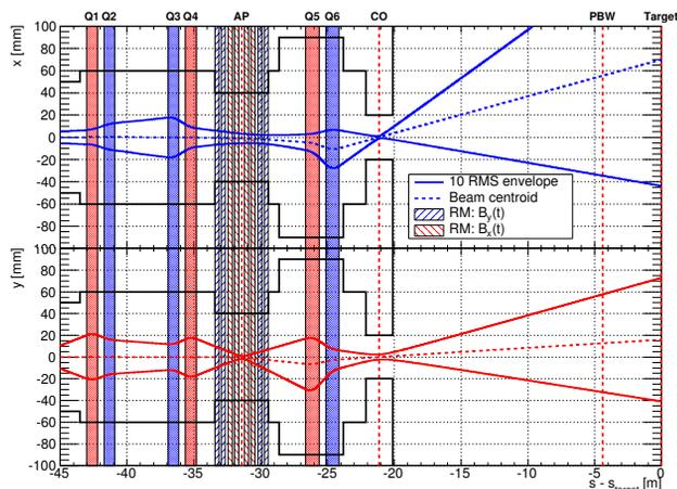
Figure 1: The final 45 m of the HEBT before the target surface. The optics are shown at maximum deflection.
