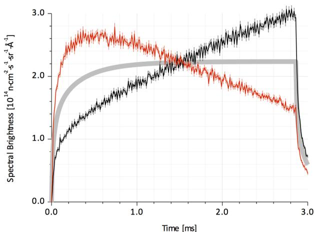
Figure 2: One example of an alternative scanning scenario. The beam is rastered vertically at 29 kHz and swept once horizontally during the 2.86 ms pulse. Thermal neutron pulses (0.8 Å) from upstream (red) and downstream (black) moderators are shown with the reference output from a square proton pulse shown in grey.
