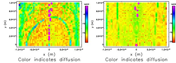
Figure 7: Comparison of frequency map analysis shows that the quasi-third-order achromat scheme (right figure) has better performance.
