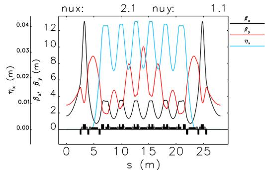
Figure 1: Twiss parameters in a 7BA arc cell with a length of 27.2 m. Natural emittance is 150 pm at a beam energy of 6 GeV. The black curve denotes horizontal beta function; red curve, vertical beta function; blue curve, horizontal dispersion function.
