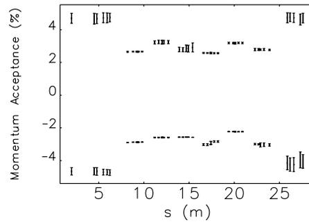
Figure 4: Local momentum acceptance with 50 ensembles of errors (random, systematic magnetic errors, and tilt errors on quadrupoles and sextupoles). Tracking is performed at locations next to each magnet in one 7BA arc cell (28 m).
