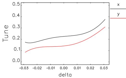
Figure 2: Horizontal (black curve) and vertical (red curve) betatron tune as a function of momentum offset  $\Delta E/E$ , dominated by third-order chromaticity.
