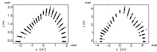
Figure 5: Comparison of dynamic acceptance shows that the quasi-third-order achromat scheme (right figure) has better performance.
