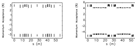
Figure 6: Comparison of local momentum acceptance shows that the quasi-third-order achromat scheme (right figure) has better performance.
