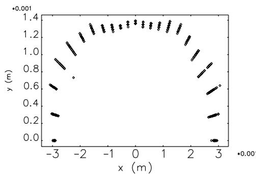
Figure 3: Dynamic acceptance with 50 ensembles of random, systematic, and tilt errors on quadrupoles and sextupoles. Tracking is performed at the center of the short straight section where  $\beta_x = 4$  m,  $\beta_y = 1.2$  m.
