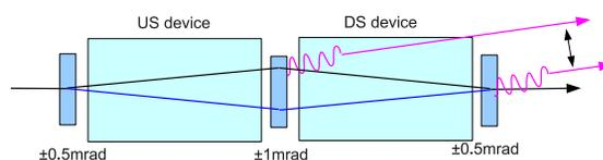
Figure 2: Diagram showing a position shift during ID switch in a triangular-bump configuration.
