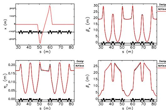
Figure 8: Lattice functions and orbit for two sectors around the ID straight section for an antisymmetric 4-corrector bump. No bump and negative bumps are shown. The order of the plot is the same as in Figure 4.
