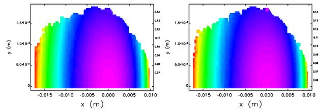
Figure 5: Dynamic aperture for the lattice without orbit bump (left) and with W-bump (right), color coding is horizontal tune.
