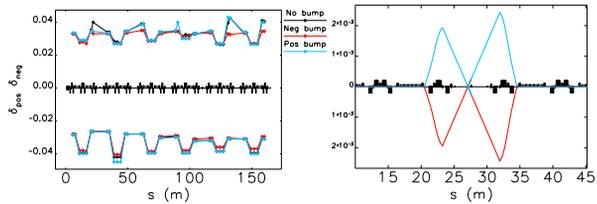
Figure 6: Local momentum aperture for lattice with W-bump.
