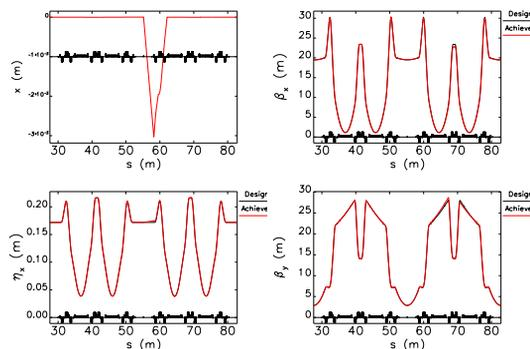
Figure 9: Lattice functions and orbit for two sectors around the ID straight section for an asymmetric 3-corrector bump. No bump and negative bumps are shown. The order of the plot is the same as in Figure 4.
