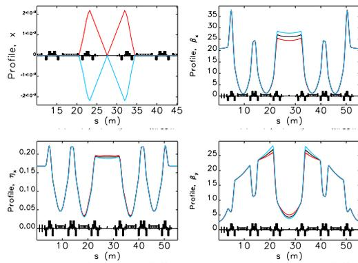
Figure 4: Lattice functions and orbit for two sectors around the ID straight section for W-bump. Starting from top left in clockwise order: orbit, horizontal beta function, vertical beta function, and horizontal dispersion. No bump, positive, and negative bumps are shown.
