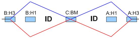
Figure 3: Five-kicker bump that allows photon beams to be sent from both undulators along the same line.
