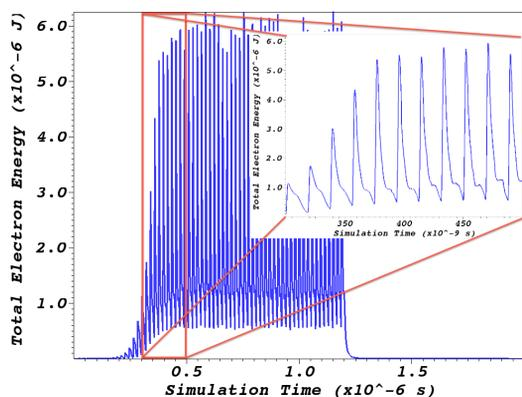
Figure 1: Total energy of the electron cloud as a function of simulation time. Bunch crossings punctuate the electron energy, which then relaxes as electrons are absorbed by the beam pipe walls.
