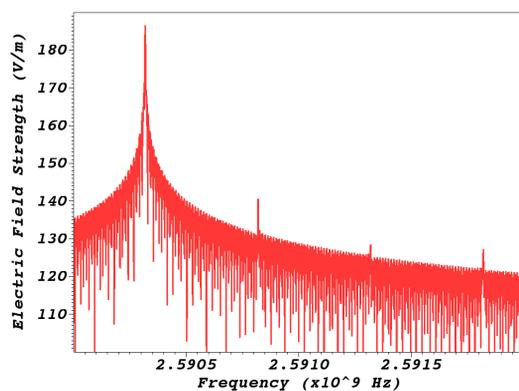
Figure 3: Simulated spectrum for integrated plasma dielectric model, where the 3-Dimensional electron densities from kinetic simulations determines the plasma dielectric strength.
