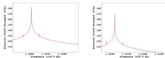
Figure 2: Synthetic spectra generated by harmonic modulation of plasma dielectric tensor. Left plot shows the spectrum with zero applied magnetic field, driven at 50% above the cutoff frequency. Right plot shows the spectrum with excitation of the extraordinary wave, near the cyclotron resonance with an applied dipole field of 0.06 T, and hence the upper hybrid resonance, driven at 5% above the cutoff frequency.
