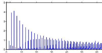
Figure 1:  $\text{Re} Z(k)$  in ohms for ANKA parameters, vs.  $k = 1/\lambda$  in  $\text{cm}^{-1}$ .
