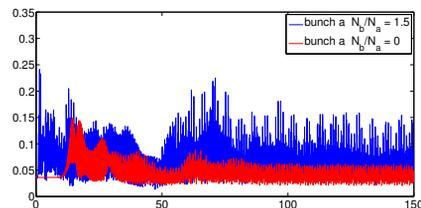
Figure 9: Power from trailing bunch (a), with and without leading bunch, which has 50% more charge.
