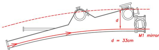
Figure 3: Vacuum chamber of CLS at dipole where IR is extracted
