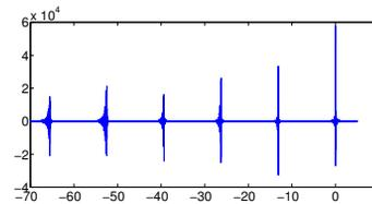
Figure 5: Wake potential for CLS model with  $d = 33\text{cm}$ .
