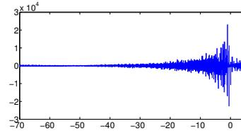
Figure 4: Wake potential  $W(z)$  in V/pC from impedance of Fig. 1., vs.  $z$  in cm.
