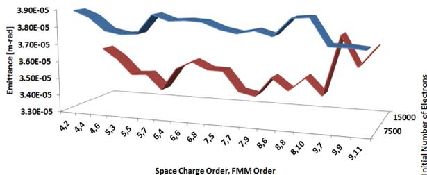
Figure 3: Final emittances [m-rad] after 1 turn vs. Space Charge Order, FMM Order using the fast multipole method.
