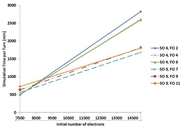
Figure 4: Simulation time per turn [mins] vs. initial number of electrons for select space charge orders, FMM orders using the fast multipole method.
