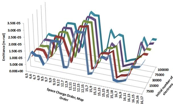
Figure 1: Comparison of Final Emittance [m-rad] vs. Space Charge Order, Map Order vs.  $N_p$  using the moment method for the UMER model.
