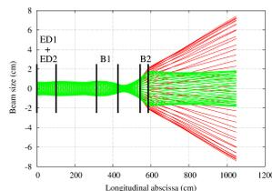
Figure 8: Axial beam envelope vs the longitudinal abscissa along the injection trajectory: the green and red curves show the result when a 0.68 kG/cm or 0 kG/cm gradient is applied to the magnet B2, respectively. The difference between the two envelopes is observed after dipole magnet B2.
