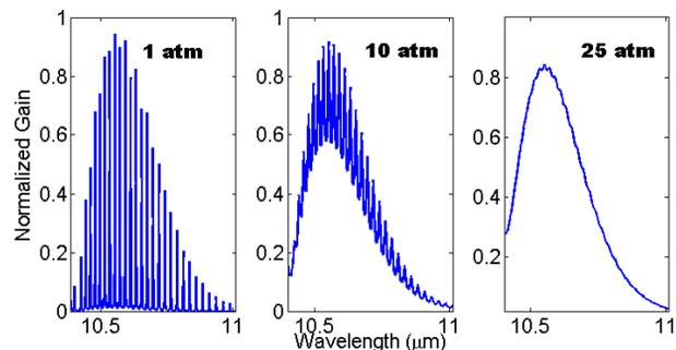
Figure 1: Simulations of the CO<sub>2</sub> gain medium at 1, 10 and 25 atm of pressure for the 10P branch.
