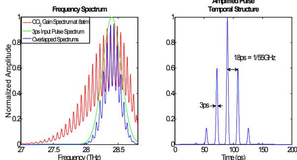
Figure 2: Simulations showing the production of a ps pulse train after amplification of a single ps pulse in a 10 atm  $\text{CO}_2$  laser.
