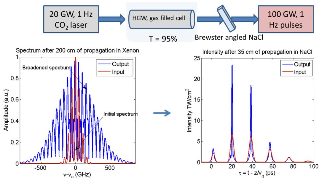
Figure 5: Top: Proposed set-up to use self-phase modulation followed by compression in NaCl to produce 100 GW CO<sub>2</sub> laser pulses. Bottom: Simulated frequency and time domain representations of our pulse train before and after the pulse compressor.
