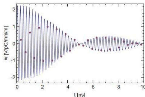
Figure 5: The time domain transverse wakefield in the SLAC s-band cavity.
