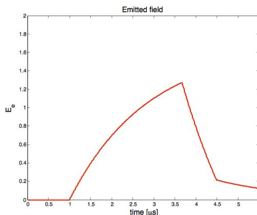
Figure 4: Temporal shape of the SLEDED pulse in the s-band cavity.
