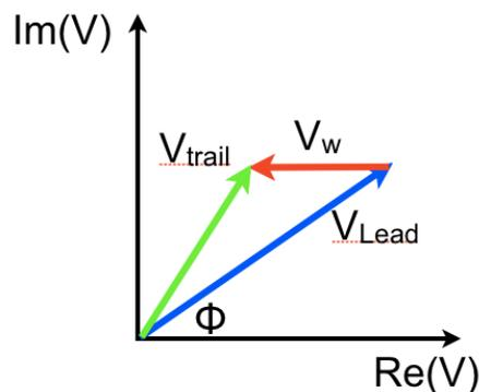
Figure 2: Phase diagram showing the RF voltage and phase difference seen by the trailing bunch.
