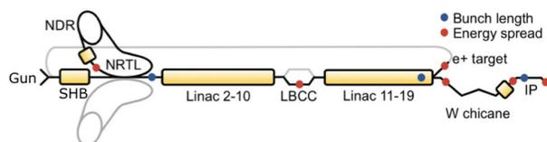
Figure 1: Overview of Linac with affected subsystems and diagnostics for multi-bunch operation.
