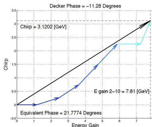
Figure 3: FACET front-end chirping scheme. Each phase arrow represents one sector and is an integer multiple of the Decker Phase.
