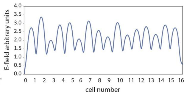
Figure 5: Bead pull field profile measurement in the 16 cell PBG structure.
