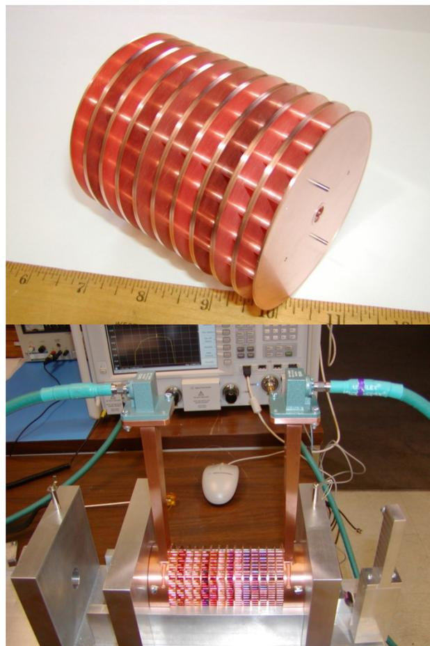
Figure 3: Photographs of the electroformed 11.7 GHz PBG cells and the assembled 16 cell PBG structure on a cold test bench.
