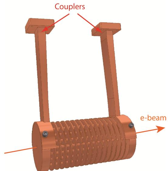
Figure 1: A 16-cell traveling-wave PBG accelerator structure with two waveguide couplers.
