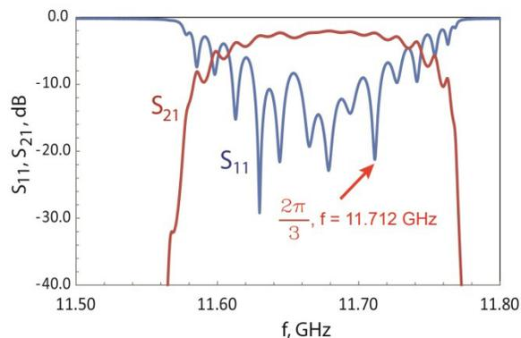
Figure 4: Transmission and reflection through the assembled 16 cell PBG structure.
