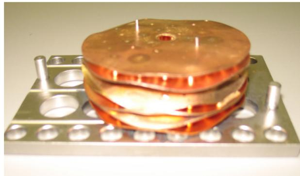
Figure 2: Photograph of the electroformed cells destroyed by brazing.
