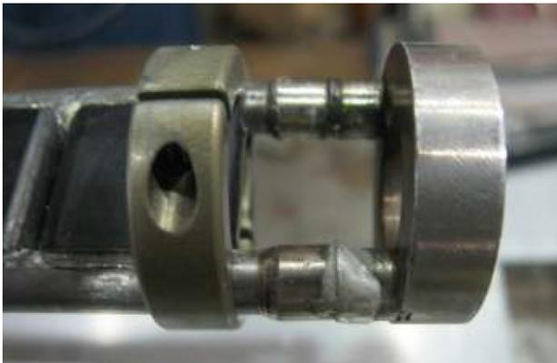
Figure 4: A downstream cooling water turn-around end of NuMI target NT-06 that failed after 4 month of operation at peak beam power of 340kW (total of  $1.3 \times 10^{20}$  protons on target, 2011, courtesy J.Hylen, Fermilab)
