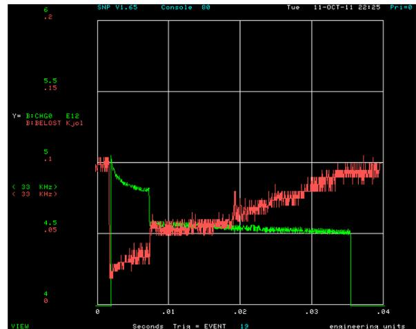
Figure 3: Losses in 8 GeV Fermilab Booster during its 15 Hz cycle occur at injection due to poorly captured beam, at the moment of notch creation (gap for extraction created with a kicker, particles lost in a gradient magnet). slow losses at high-energy (due to optics issues, RF variation), and losses at the transition energy (courtesy of Fermilab's Proton Improvement Plan team).
