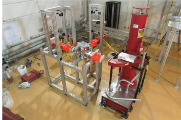
Figure 4: klystron, circulator and loads.
