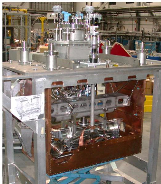
Figure 2: Injector cryomodule internal assembly.
