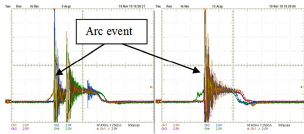
Figure 6: Examples of an arc event which did not result in a failure (Figure 6a) and one that did (Figure 6b).
