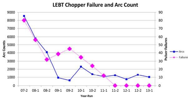
Figure 5: LEBT high voltage pulse generator MOSFET failures and arc events verses run cycle.
