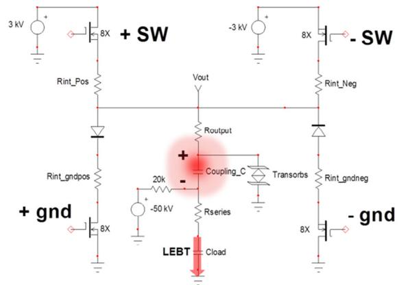
Figure 7: Simplified Schematic demonstrating an arc in the LEBT Structure and voltage reversal on the Coupling Capacitor.
