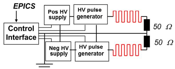
Figure 10: Block diagram of MEBT chopper system.
