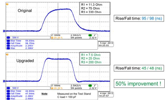
Figure 9: LEBT high voltage pulse generator rise/ fall time improvement chart.
