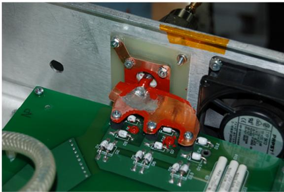
Figure 12: Matching 50 Ohm output impedance.
