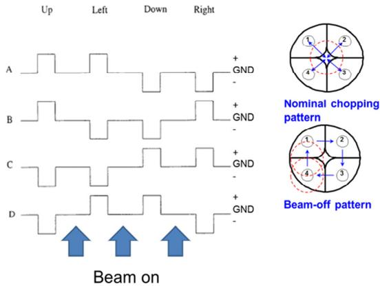
Figure 3: Four phase timing of LEBT chopper.
