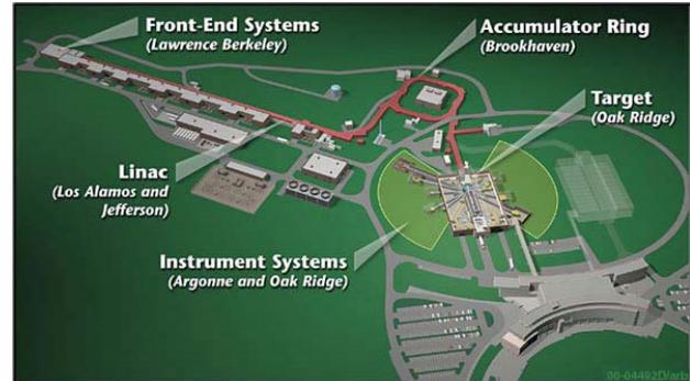
Figure 1: Layout of the Spallation Neutron Source in Oak Ridge, TN.
