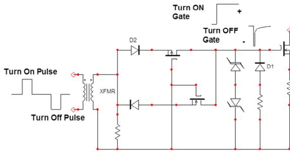
Figure 8: Gate drive schematic.
