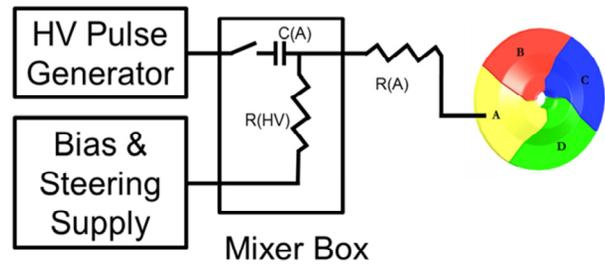
Figure 4: Block diagram of one channel of the LEBT chopper system
