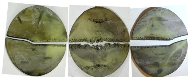
Figure 7: Three circular cross section cut-outs of the inner, front facing surface of target number 4 vessel – with a clear cavitation induced cut-through on the mid-plane.
