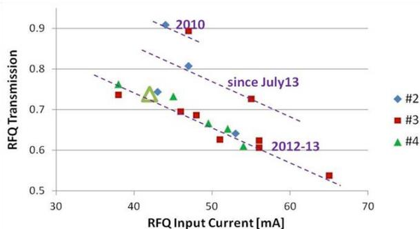
Figure 3: RFQ beam transmission as a function of input beam current indicating reduced transmission during the 2012-2013 detuned RFQ operation.
