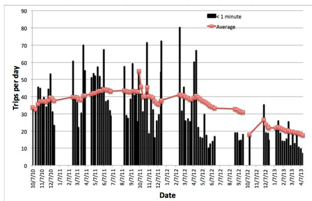
Figure 6: Short duration trip frequency (typical of warm linac RF faults) history at SNS.
