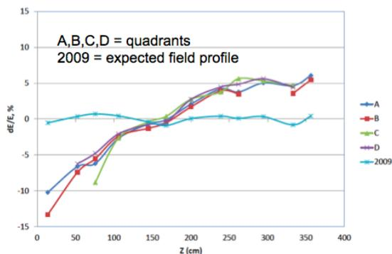
Figure 4: Field distribution along the SNS RFQ in 2012-2013 run.
