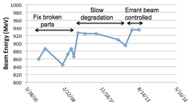
Figure 5: Operational linac output beam energy, indicating a period of performance degradation in 2009-early 2011.
