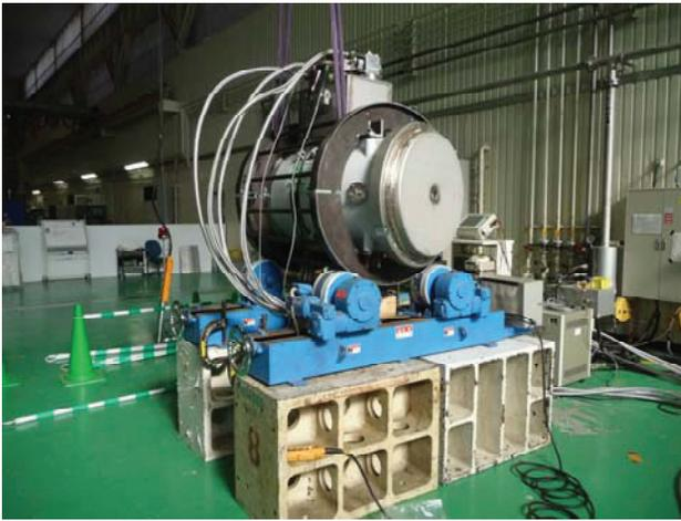
Figure 9: Picture of the test bench during rotation tests of the model superconducting-magnet.
