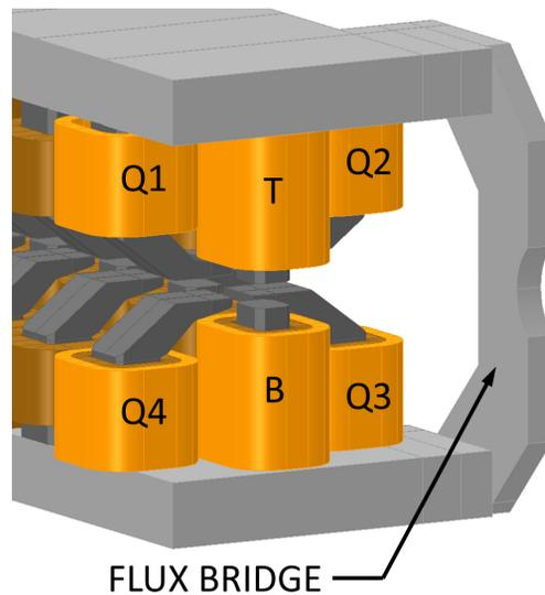
Figure 3: Configuration of the upstream corrector coils.
