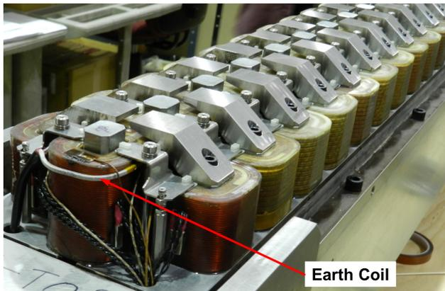
Figure 2: Top jaw coil and pole configuration. The centered vertical field poles alternate with pairs of horizontal poles along the undulator axis. The bottom jaw configuration mirrors this arrangement.
