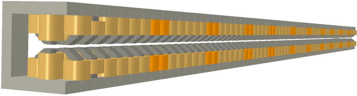
Figure 5: IEX undulator quasi-periodic pole positions.
