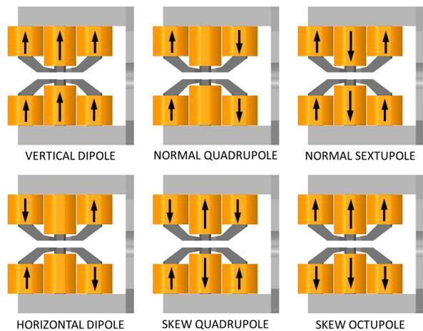
Figure 4: Coil field directions for the various multipole moments.
