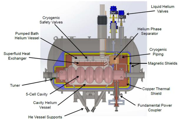
Figure 1: Layout of the 704 MHz SRF cryomodule.
