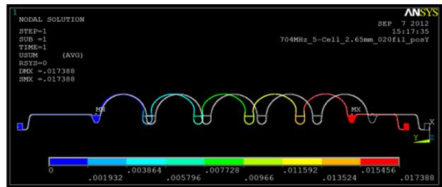
Figure 5: Relaxed and deformed shapes of the cavity.
