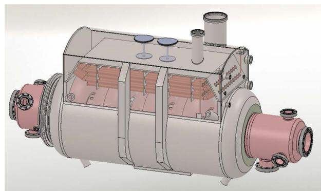
Figure 2: Layout of the 704 MHz cavity in a helium vessel.
