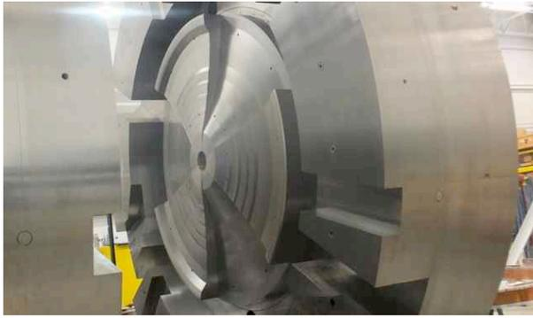
Figure 2: The machined sector cyclotron pole pieces on the 2.2-m diameter pole for the magnet. The coil cryostat is in the slot between the pole and the return iron yoke.
