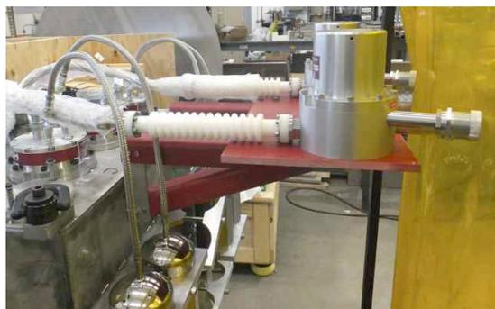
Figure 5: The coolers mounted on the coil current.
