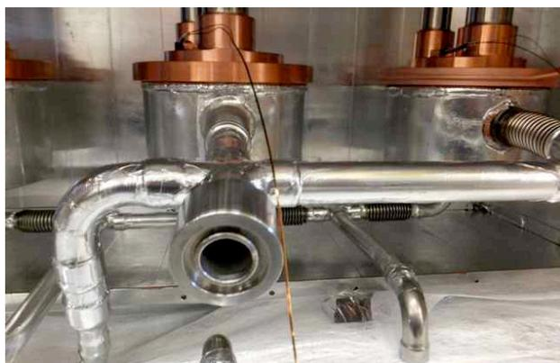
Figure 6: The condenser heat exchangers for two of the three coolers. Warm gas from the magnet enters the condenser from the top. Cold gas leaves from the condenser bottom.
