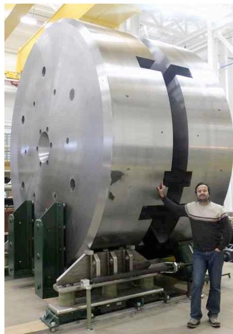
Figure 1: The split magnet iron return path and poles.
