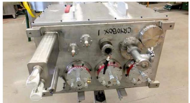
Figure 4: The top of the coil 1 turret cryobox showing the cooler cold heads (labeled A, B, and C), the current leads, the instrumentation plugs, and the safety vent tubes.
