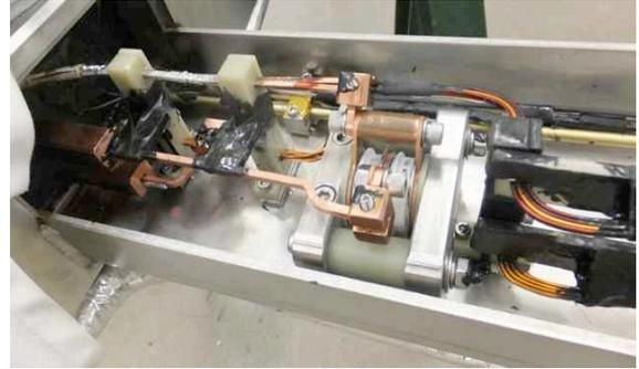
Figure 3: Quench Si diode assembly in the cryostat neck.
