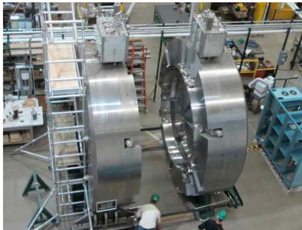
Figure 7: The magnet coil mounted in the cyclotron gas stopper magnet iron return yoke.
