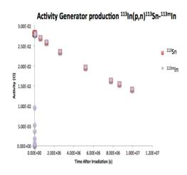
Figure 1: Activity of parent  $^{113}$ Sn and daughter  $^{133m}$ In produced from the generator reaction.
