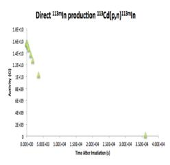
Figure 2: Activity of <sup>113</sup>In produced from the direct reaction.
