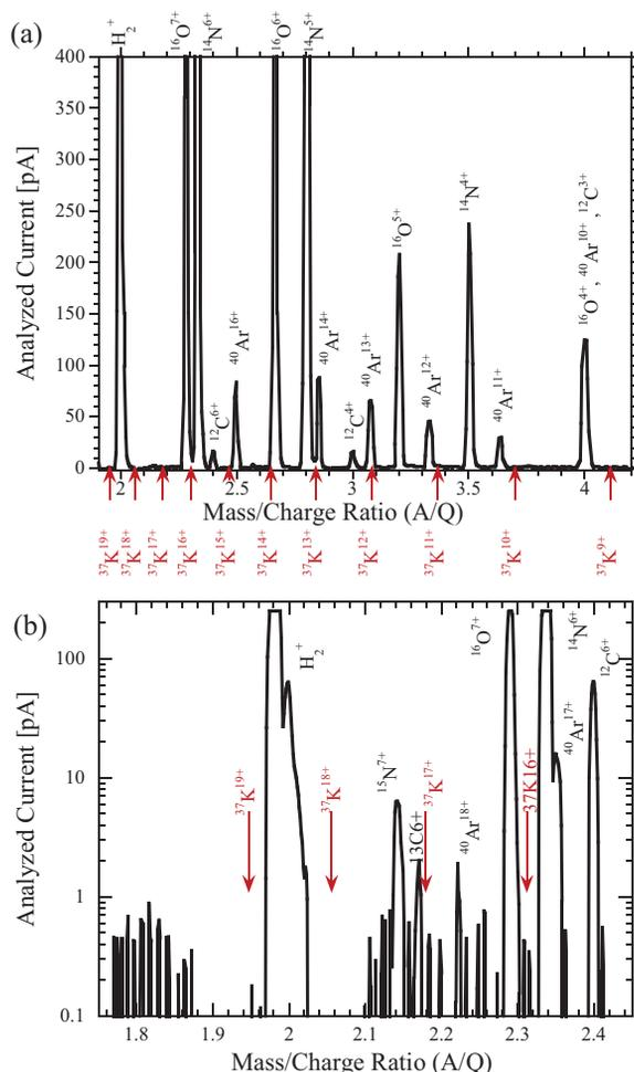
Figure 7: (a) Charge state distribution of the residual ion beam from the EBIT where the position of various  $^{37}\text{K}^{n+}$  ions are indicated. (b) High resolution, high sensitivity A/Q scan, charge states for  $^{37}\text{K}^{16+ - 19+}$  ions are indicated.
