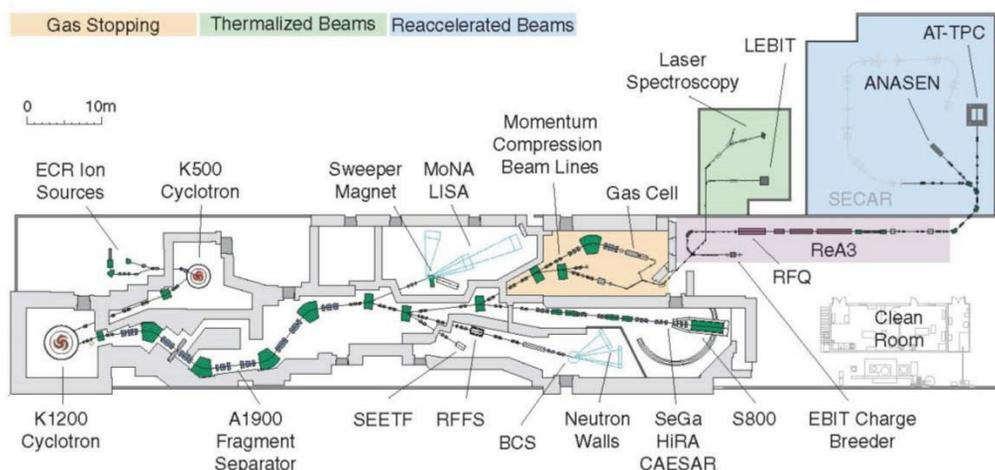
Figure 1: Facility layout of the National Superconducting Cyclotron Laboratory with the Coupled Cyclotron Facility and the newly commissioned gas stopping area and reaccelerated radioactive ion beam capabilities[5].
