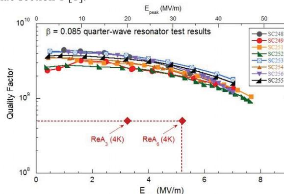
Figure 9:  $Q_0$  vs.  $E_{\text{acc}}$  ( $V_a/\beta\lambda$ ) curves measured during vertical acceptance tests of the  $\beta=0.085$  ReA3 cavities at a temperature of 4.2 K.
