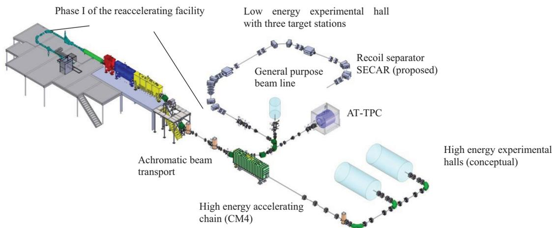
Figure 2: Layout of the ReAccelerator facility and the transport lines into the low energy experimental hall. In addition, the first cryomodule of the high energy section of the linac is shown.
