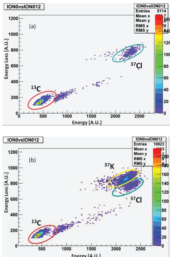
Figure 8: Particle identification (PID) obtained with the ANASEN ionization chamber. (a) PID without injection radioactive  $^{37}\text{K}$  into the EBIT (b) PID when radioactive  $^{37}\text{K}$  is injected into the EBIT.
