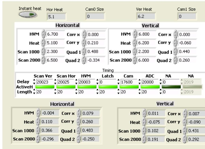
Control of accelerating voltages, cathode current, deflector voltages, magnets and timing.
