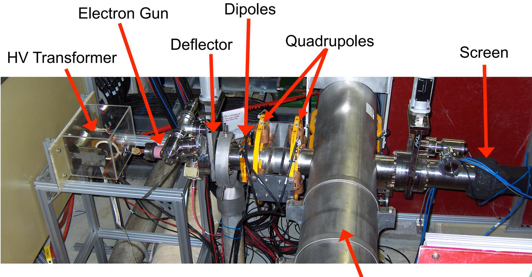
*Electron scanner now covered with magnetic shield*
