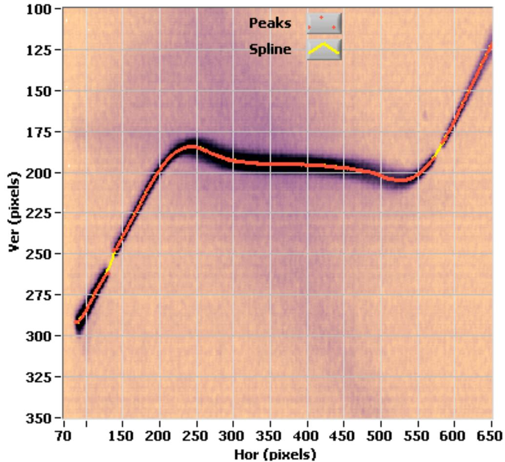
Overlay of camera image with peaks and spline fit
