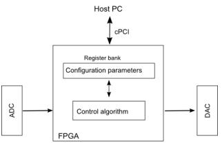
• The register bank can be expanded to 2<sup>15</sup> 16-bit registers:
