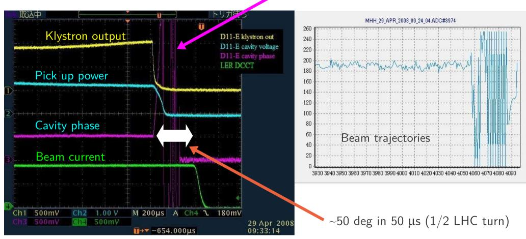
Abrupt phase changes  $\rightarrow$  corresponding orbit changes and beam losses
