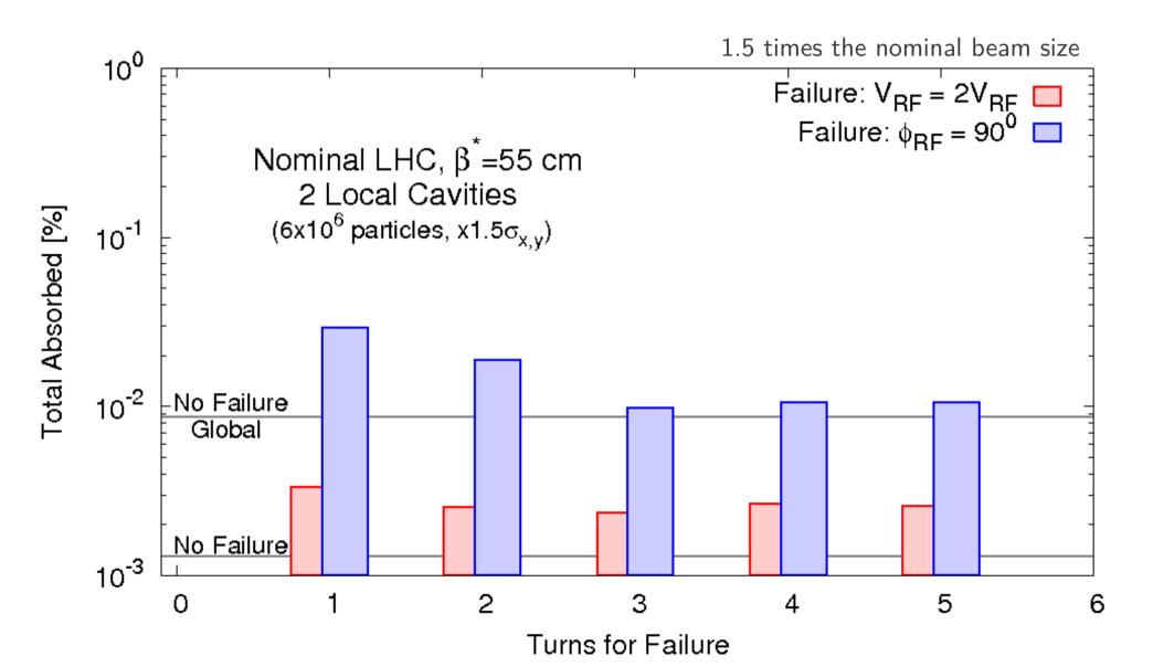
% Lost Due To  $90^{\circ}$   $\phi$ -Failure
