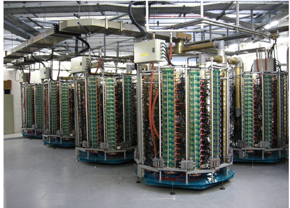
180 kW 350 MHz solid state amplifier, each column 45 kW (Soleil)
