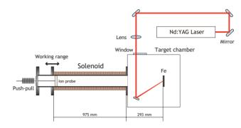
Figure 1: LIS experimental setup sketch. The push-pull allows the ion probe to be moved along the beam axis.
