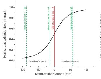
Figure 3: Normalized magnetic distribution around the end of solenoid (red line) and three scanned positions of the beam axis (green dash lines).
