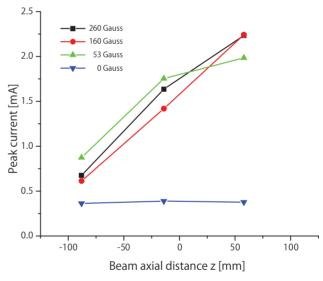
Figure 5: Peak current for magnetic field strength vs beam axial distance. No magnetic field represents blue line and that is constant for z position.
