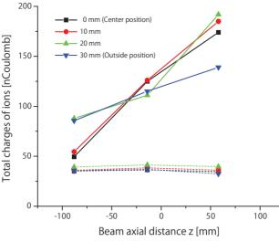
Figure 4: These lines show total ion charges for radial position with beam axial distance. Solid lines are for maximum magnetic field of 260 Gauss and dash lines are for no magnetic field. Each color represent a radial position from the center of beam.
