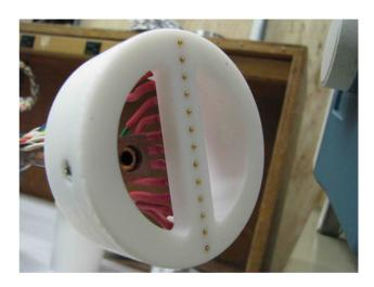
Figure 2: The ion probe with bias voltage can measure the ion current distribution simultaneously for 13 radial positions.
