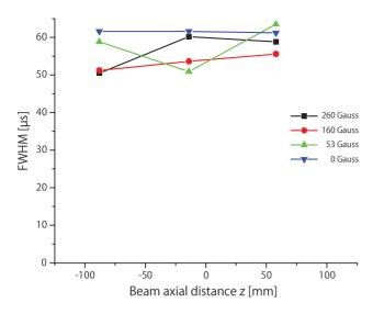
Figure 6: FWHM of beam pulse length for magnetic field strength vs Axial position. The results show no dependence on field strength.
