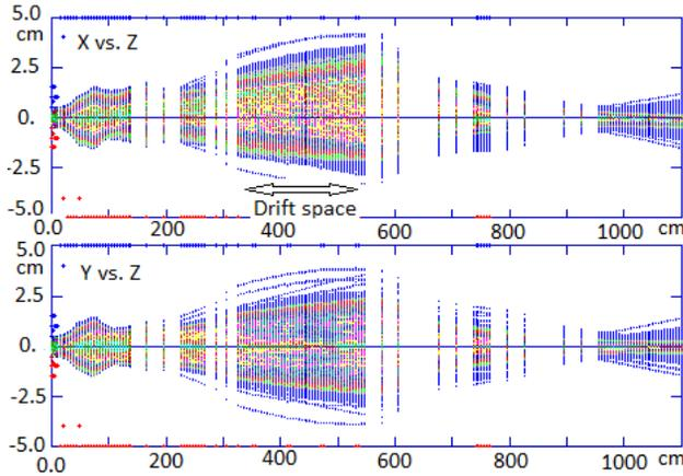
Figure 5: Beam envelope vs. Z. The drift space shown is the compression section between the 3<sup>rd</sup> harmonic cavity and booster linac.
