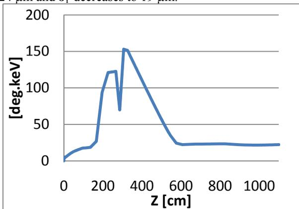
Figure 7: Longitudinal emittance vs. Z.
