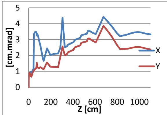
Figure 6: Emittance vs. Z. The final emittance is 33  $\mu\text{m}$  in X direction and 24  $\mu\text{m}$  in Y direction.
