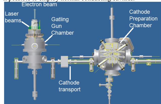
Figure 4: Cathode preparation chamber and gatling gun chamber
