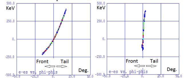
Figure 3: Optimized longitudinal phase space after bunching cavity and 3<sup>rd</sup> harmonic cavity (Left, reference energy: 840 keV) and at booster linac exit (Right, reference energy: 8.5 MeV).
