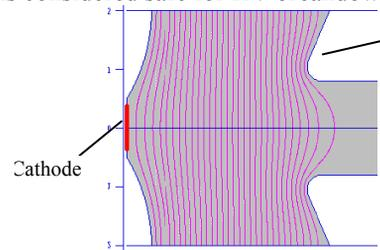
Figure 2: Individual cathode. The gap between cathode and anode is 3 cm.
