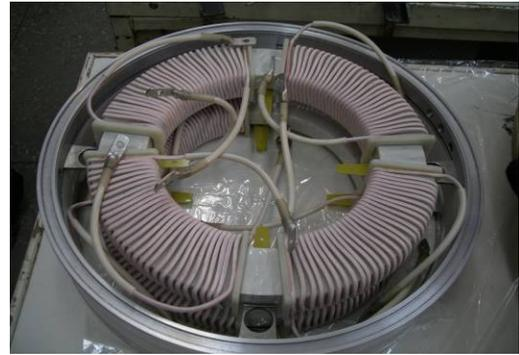
Figure 5: Prototype of the transformer section.
