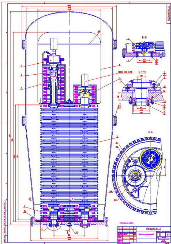
Figure 3: High voltage terminal with electron gun and collector inside the pressure vessel.
