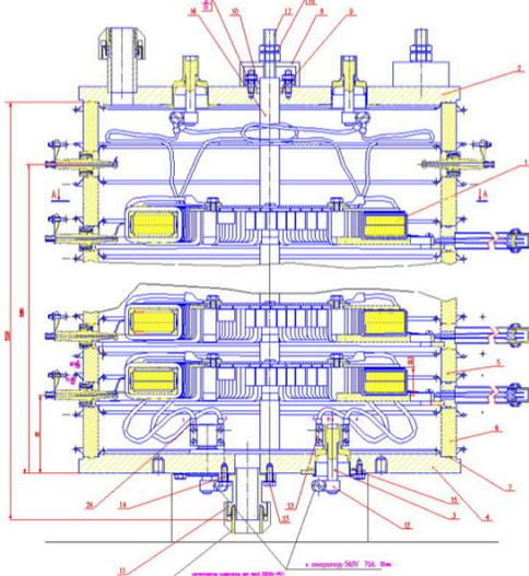
Figure 4: High power cascade transformer.
