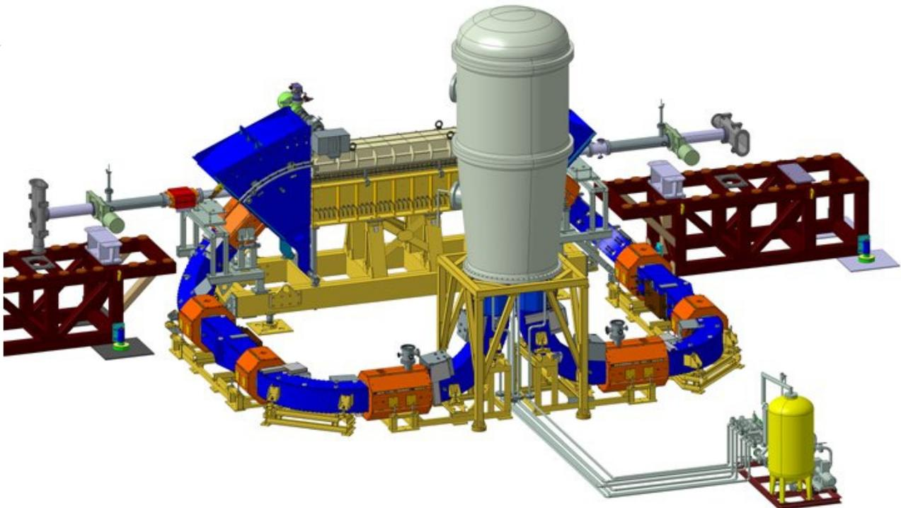
Figure 1: Layout of the 2 MeV electron cooler for COSY.
