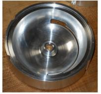
Figure 7: Cavity side of a machined DSRL half-cell.
