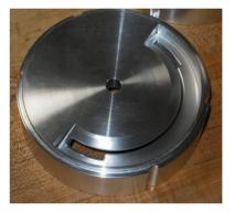
Figure 8: Void side of a machined DSRL half-cell.
