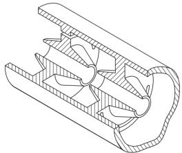
Figure 1: Slot resonance linac structure. Each slot extends nearly 180° in azimuth.
