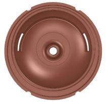
Figure 5: Solid model drawing of the cavity side of the end cell. The wall rounding was offset from the center axis compensate the perturbation in the magnetic field caused by the asymmetric slot geometry at the ends of the linac.
