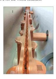
Figure 8: Piston Tuners in ReA3-RFQ.
