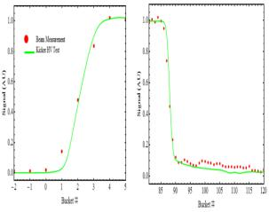
Figure 5: Gap Clearing Kicker rise and fall time measurements. The horizontal scale is in 53 MHz buckets and the vertical scale is in arbitrary units. The red trace is the beam measurements and the green trace is the integrated magnetic field calculated from the kicker voltages. The Kicker Rise and Fall times are within 57 nsec as specified.
