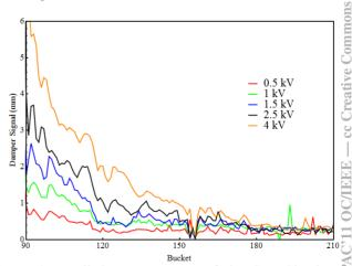
Figure 6: Detailed measurements of the Gap Clearing Kicker tail. The vertical scale is the measured kick in mm and the horizontal scale is in 53 MHz buckets. The different traces correspond to different kicker excitation levels.
