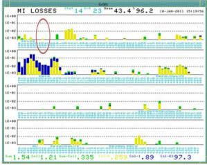
Figure 7: Main Injector loss plot with the Gap Clearing Kicker OFF (top) and ON (bottom). The vertical axis is the integrated loss at each MI beam loss monitor at the end of each cycle (in log scale). The yellow color indicates the contribution to the total loss from injection, the blue from the losses during acceleration and the green from extraction.
