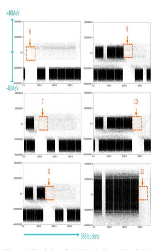
Figure 1: Simulation of multi-batch slip stacking in Main Injector. After 5 Booster batches have been decelerated there some left over beam in the gap where the rest of the 11 batches are injected (red squares).
