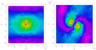
Figure 4: Electrical (at the left) and magnetic (at the right) fields modulus in a rectangular chamber of 6x6 mm<sup>2</sup> cross-section of a helical undulator with left helicity.
