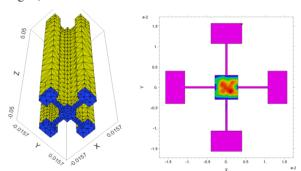
Figure 2: 3D mesh for the vacuum chamber used in modeling. At the right: The modulus of electric field for the chamber at one particular moment (frame from a movie).
