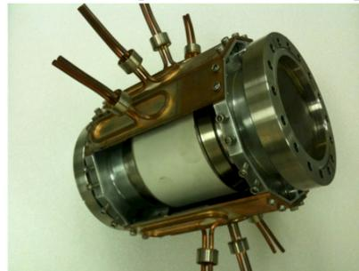
Figure 1: Ceramic break with ferrite HOM damper.
