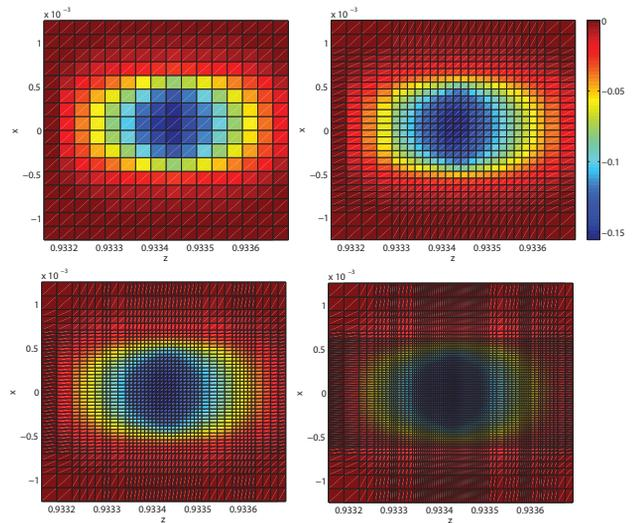
Figure 4: Meshes with increasing density obtained with the new algorithm for the bunch shown in Figure 2.
