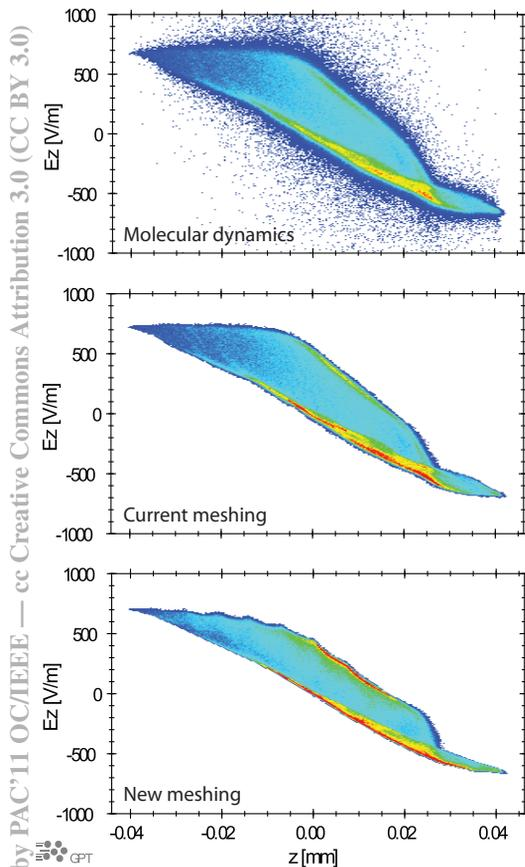
Figure 3: GPT simulations with various space-charge models corresponding to Figure 2.
