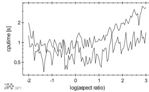
Figure 1: CPU time for the current (top line) and new (bottom line) meshing scheme.
