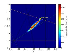
Figure 3: Tune spread plot calculated at 1000 turn after the sextupole field rampings
