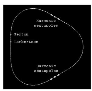
Figure 1: Locations of the septum, Lambertson, and harmonics sextupoles in the Debuncher ring.
