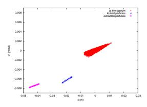
Figure 4: Phase space (red) at the septum with kicked (at the septum:blue) and extracted (at the Lambertson:pink) particles
