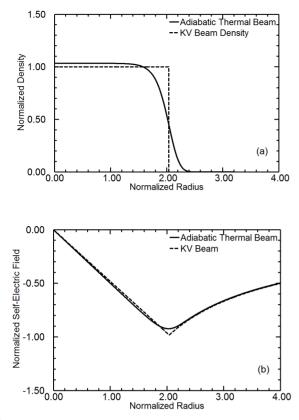
Figure 1: Plots of a) normalized density  $n_b / n_{KV}(0,0)$  and b) normalized radial self-electric field  $S^{3/2}KE_r / 4\varepsilon_{th}^{1/2}qN_b$ versus normalized radius  $r/\sqrt{4\varepsilon_{th}S}$  in the KV-type beam equilibrium (dashed curve) and the adiabatic thermal beam equilibrium (solid curve) at s = 0 for the same choice of system parameters as in Fig. 1. Here,  $n_{KV}(0,0)$ is the density of the KV-type beam equilibrium at s = 0and r = 0
