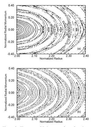
Figure 3: Close ups of Poincare surface-of-section maps of charged-particle trajectories for the two cases shown in Fig. 2.
