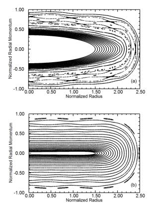
Figure 2: Poincare surface-of-section maps of chargedparticle trajectories in a) KV-type beam equilibrium and b) adiabatic thermal beam equilibrium for  $P_{\theta} = 0$  and the same choice of system parameters as in Fig. 1. Here, the normalized radial momentum is  $(S/4\varepsilon_{th})^{1/2} dr/ds$  and the normalized radius is  $r/\sqrt{4\varepsilon S}$
