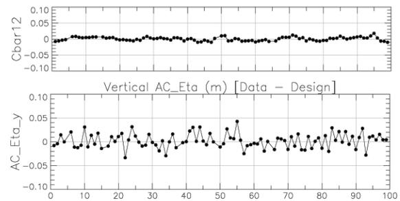
Figure 2: Measured coupling and vertical dispersion after low-emittance tuning. Horizontal axis is BPM index. RMS Cbar12 = 0.006, RMS vertical dispersion = 15mm.
