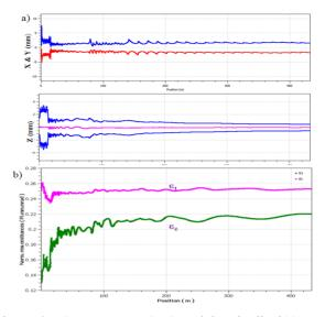
Figure 8: a) Transverse (x,y) and longitudinal(z) r.m.s. beam envelopes and (b) emittances along the SC linac in presence of failed solenoid after compensation.
