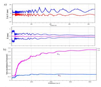
Figure 7: a) Transverse (x,y) and longitudinal r.m.s. beam envelopes and (b) emittances along SC linac in the presence of failure of the first solenoid in SSR0 section.
