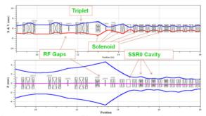
Figure 5: Beam profile in transverse plane (top) & longitudinal plane (bottom) in presence of a failed cavity after its compensation.
