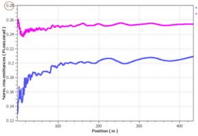
Figure. 6: Longitudinal (blue) and transverse (magenta) emittance dilution through SC linac in presence of failed cavity with compensation scheme.
