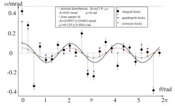
Figure 3: Correction of third integer resonances according to the previous scheme. Each set of samples (green, blue and black dot) represent one dipole segment. The green dots fit smoothly into the desired field distribution (red line). In contrast, the integral kick angles vary strongly from the desired field and a  $\chi^2/dof = 24.203$  is obtained.
