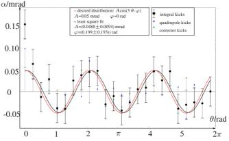
Figure 4: Correction of third integer resonances according to the new scheme. Each set of samples (green, blue and black dot) represent one dipole segment. In comparison with the previous correction, the integral kick angles fit well to the desired field (red line) and a much better  $\chi^2/dof = 0.925$  is obtained.
