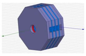
Figure 5: Solenoid for emittance compensation.
