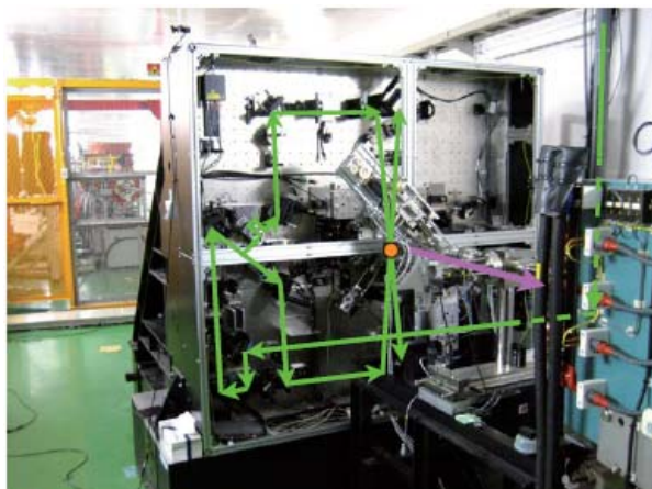
Figure 2: Main optical table of the interferometer. Green line shows the laser path of the 174^\circ mode.
